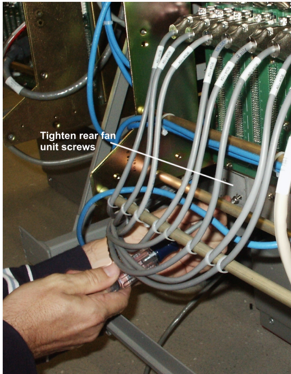
Figure 47: Tighten rear fan tray screws
