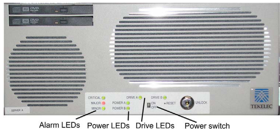
Figure 3-30 T1100 Showing Power LEDs
