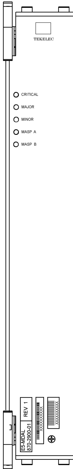
Figure A-4 E5-MDAL LEDs
