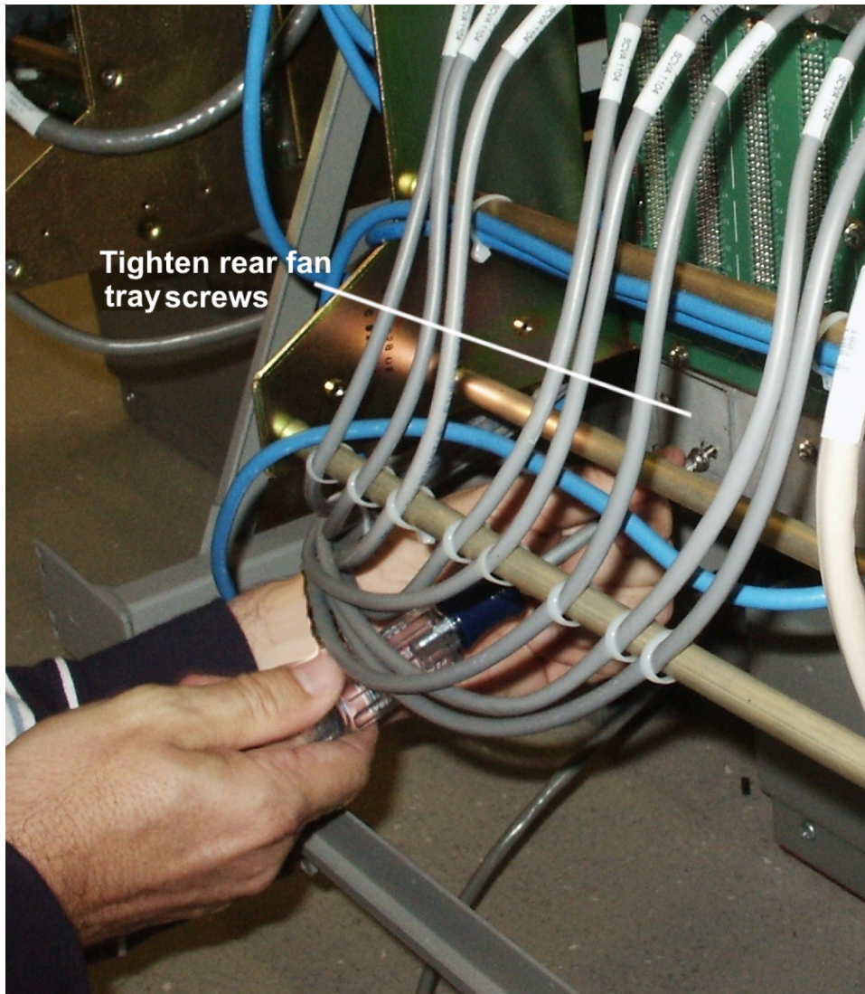
Figure 6-21 Tighten rear fan tray screws
