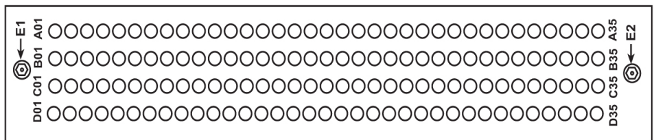
Figure B-42 Extension Shelf Backplane Pin-Outs, Bottom Connector
