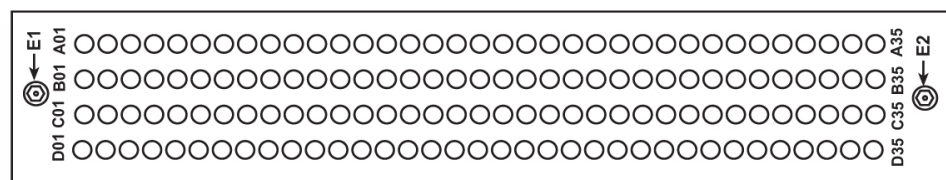
Figure B-24 Control Shelf Backplane Pin-Outs, Top Connector
