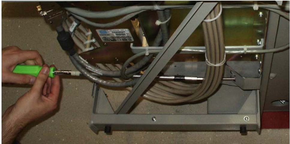
Figure 6-22 Tighten fan side bracket screws
