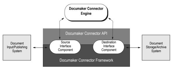
The source and destination interfaces are customizable and this chapter explains how to create new implementations of these components.
