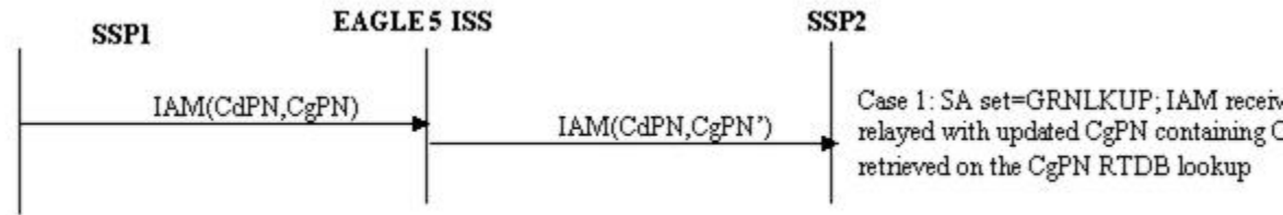
Figure 3-24 ISUP IAM Message Flows for TIF GRN for TIF CgPN Service
