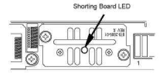
The Shorting Board LED turns green and the fuse alarm LEDs turn red.
