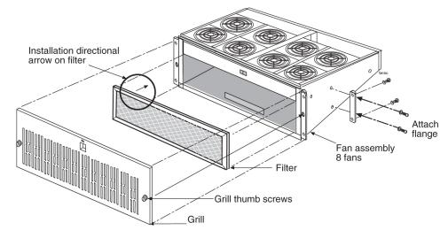
Figure 6-25 Fan Assembly with Grill and Filter
