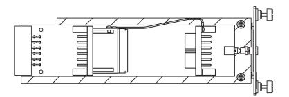
4. Slide the jumper board back into the FAP. Verify the OP/MAINT LED lights green. The fuse alarm LED returns to green.
