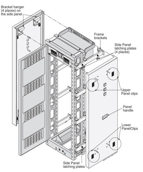
Figure 4-16 Heavy Duty Frame Panels
