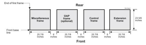
3. Align the frame isolation sheet/template (refer to Figure 4-8) along the chalk line to mark anchor location in the middle of each oval anchor slot and to mark the corners of the first frame.
