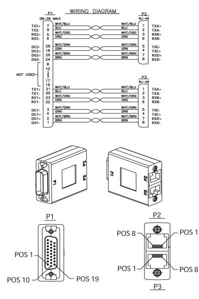
Figure C-17 DB26 Male to Dual RJ45 Adapter
