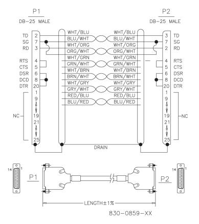
Figure C-38 Null-MODEM for Terminal
