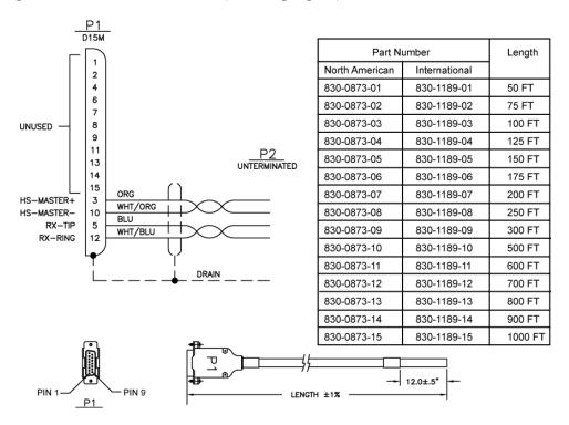
Figure C-32 Master Clock Cable (BITS/High-speed)
