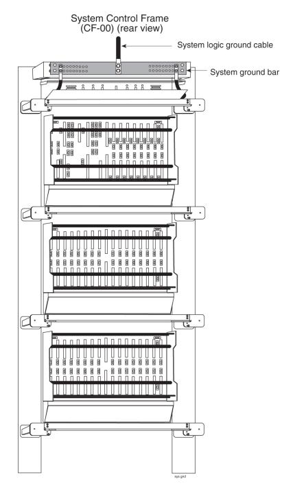
Figure 5-20 System Logic Ground Bar and Cable
