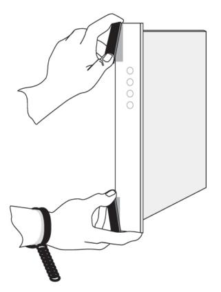
Figure 2-1 Removing a Card
