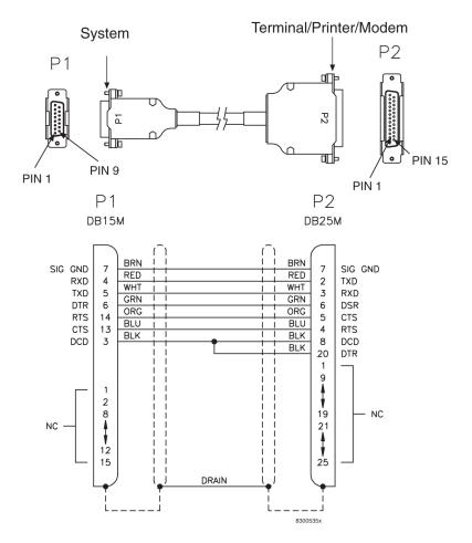
Figure C-55 Terminal/Printer Cable
