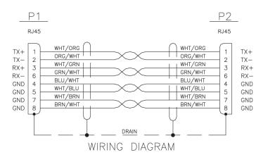
Figure C-52 Straight Through Cable (CAT-5)
