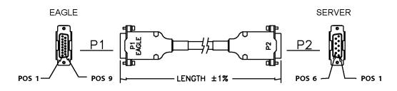
Figure C-56 Terminal Server Serial Cable with Flow Control (P/N 830-1201-xx)
