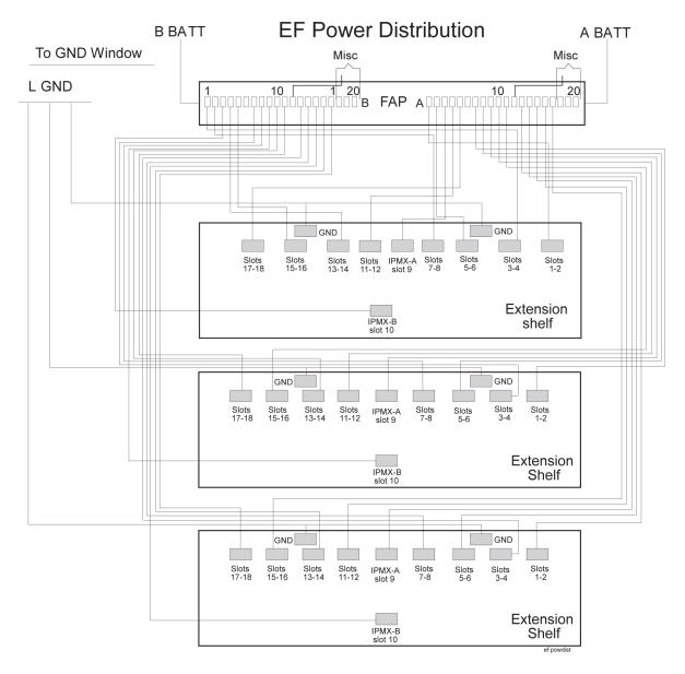
Figure 5-29 Extension Frame FAP (P/N 870-0243-08 and P/N 870-1606-xx)
