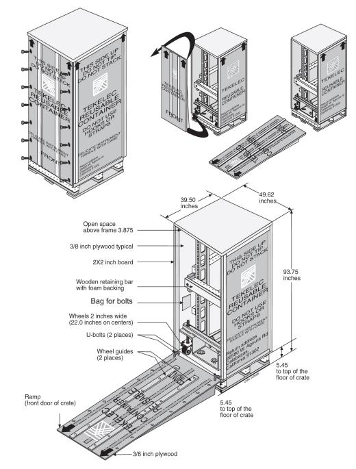
Figure 4-2 Shipping Container for Heavy Duty Frame
