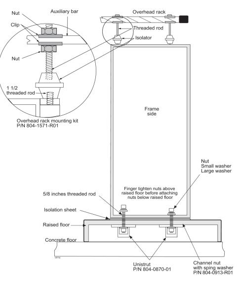
Figure 4-11 Raised Floor Installation With Unistrut
