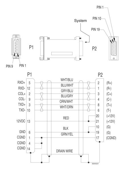
Figure C-21 ENET Adapter 15-Pin to 26-Pin (P/N 830-0425-01)
