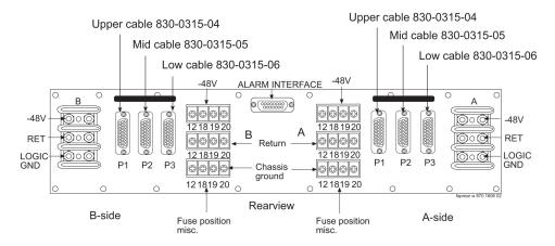
Figure 6-47 Holdover Clock FAP Connections
