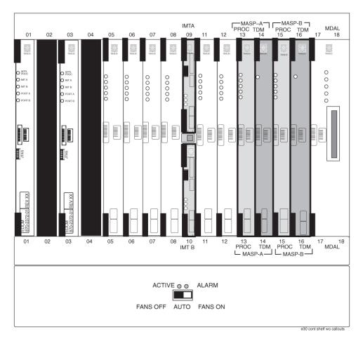
Figure 6-29 Front Card Suite with Fan Switch
