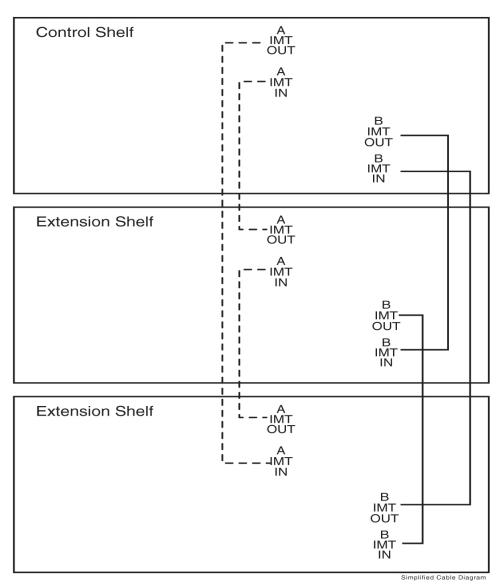
Figure 6-1 Interprocessor Message Transport Cables
