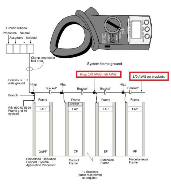
Figure 5-17 System Frame Grounding
