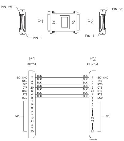
Figure C-50 Serial Interface/Modem Adapter
