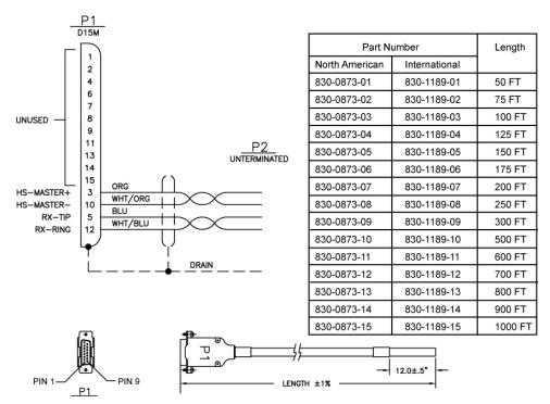
Connect P1 of the high-speed master and composite clock cable (P/N 830-0873-xx or P/ N 830-1189-xx) connector end to the appropriate IDLE ckock connector(J48 or J49). Tighten the connector with a slotted screw driver.
