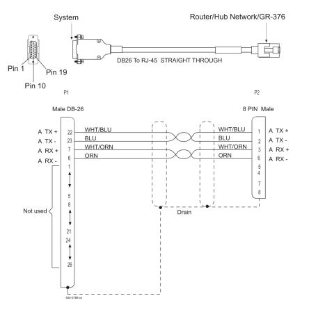
Figure C-53 Straight Through Patch Panel Cable
