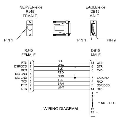
Figure C-58 Terminal/Server Serial Port Adapter, MRV (P/N 830-0915-02)
