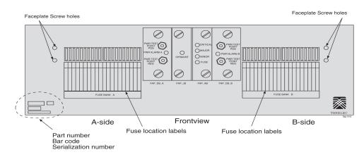
Figure 5-8 Fuse and Alarm Panel (P/N 870-1606-xx/870-2320-xx) Front
