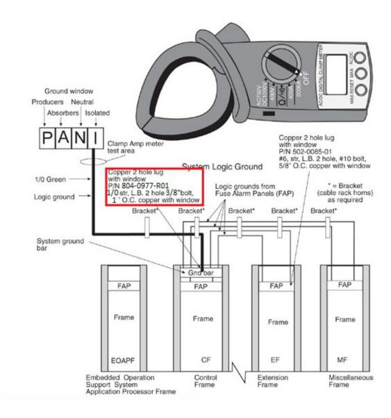
Figure 5-18 System Logic Grounding
