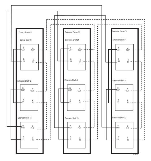
Figure 6-2 Three-Frame Configuration
