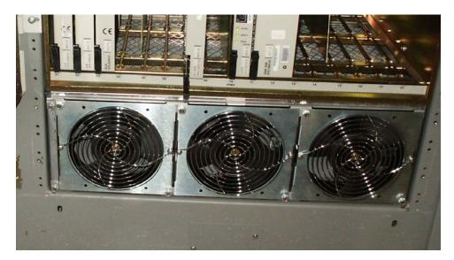
Figure 6-20 Fan tray inserted into fan tray bracket in the frame- front view
