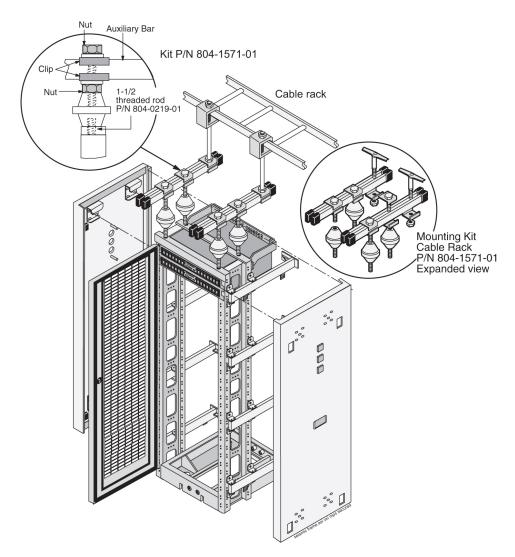
Figure 4-15 Heavy Duty Frame Installation With Cable Rack
