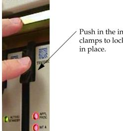
Push in the inject/eject clamps to lock the card
