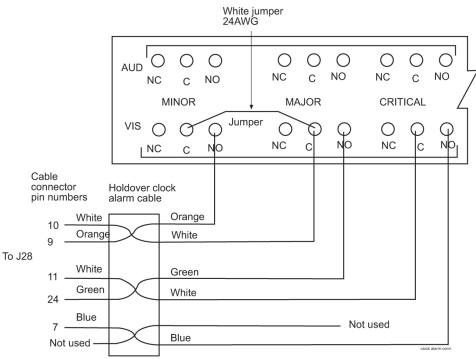
Figure 6-50 Holdover Clock Alarm Connections
