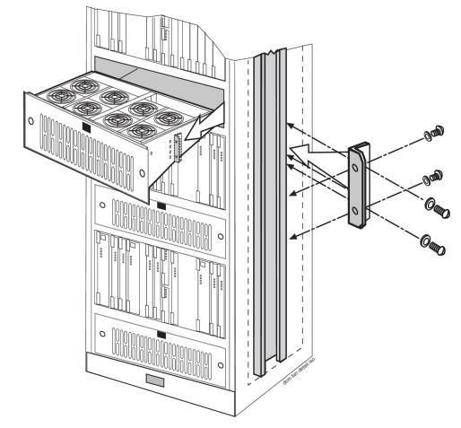
Figure 6-27 Fan Bracket Installation
