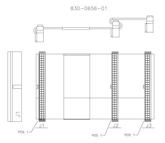
Figure C-23 Fifty Position/Hard Drive I/O Cable
