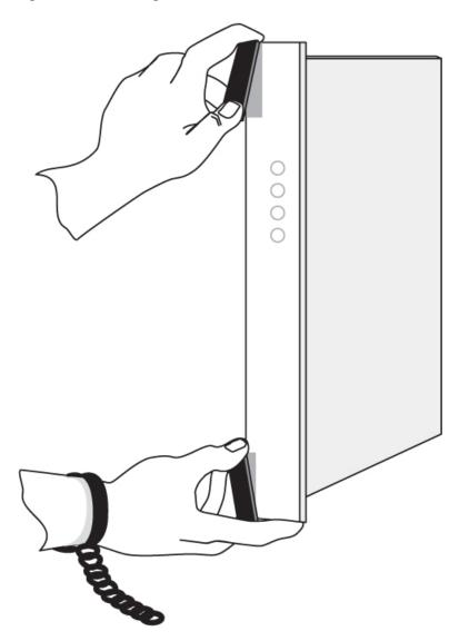
Part number, **LEDs**, text and bar code (**CLEI** and serial number) are located on the faceplate of each card. The cards in the frames are configured with specific functions and services.
