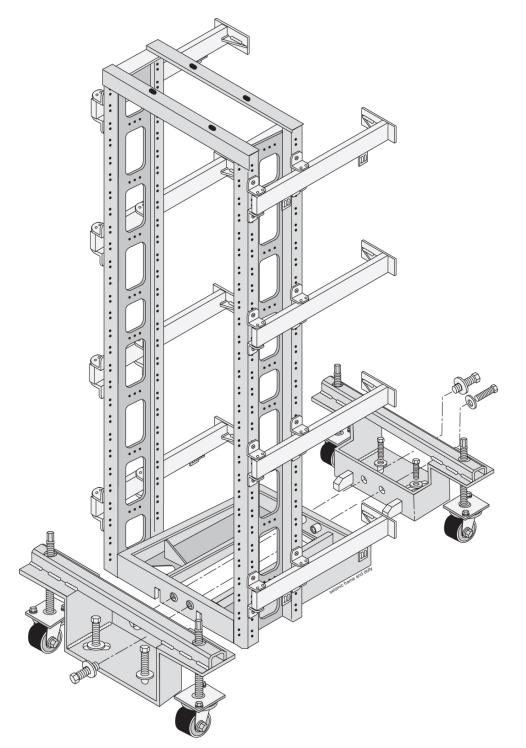
Figure 4-5 Heavy Duty Frame with Dolly
