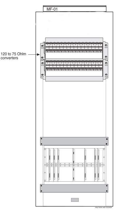
Figure 6-52 Miscellaneous Frame with 120 Ohm Converter
