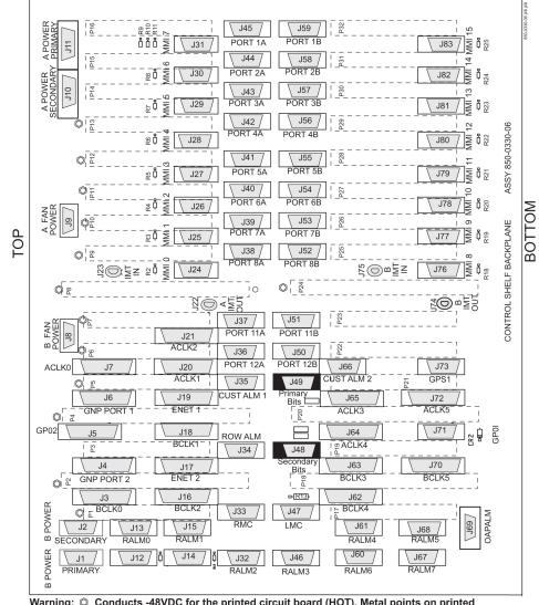
Figure 6-31 Control Shelf (P/N 850-0330-06 or -07) BITS Connectors
