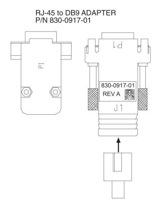
Figure C-45 RJ 45 to 9 Pin Adapter
