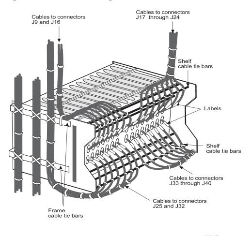
Figure 6-10 Interface Cable Routing, Extension Shelf
