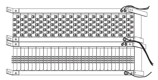
Rear 120 ohms to 75 ohms converter
