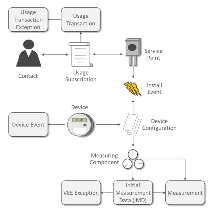
A Device represents a physical meter, communication module, or some other device out in the field. A Service Point is the point at which service is delivered to a customer and a device can be installed. The Install Event is a record of a specific device installed at a Service Point. A Contact is the customer that should be contacted in association with the Usage Subscription.
