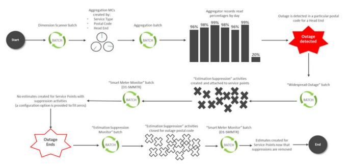
In order to determine if an area is experiencing a widespread outage, the median read percentage of prior days is used as the basis for comparison. The median was chosen instead of the average to help reduce the impact of outlier values. This is illustrated in the example below.
