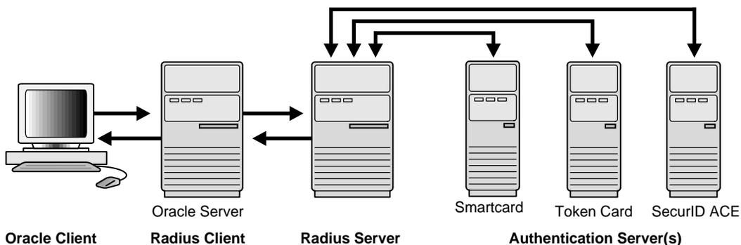
In an Oracle environment (Figure 3-1), the Oracle server acts as the RADIUS client; it passes information between the Oracle client and the RADIUS server. Similarly, the RADIUS server passes information between the Oracle server and the appropriate authentication server(s). To secure authentication information during transport, RADIUS converts it to a hash value.
