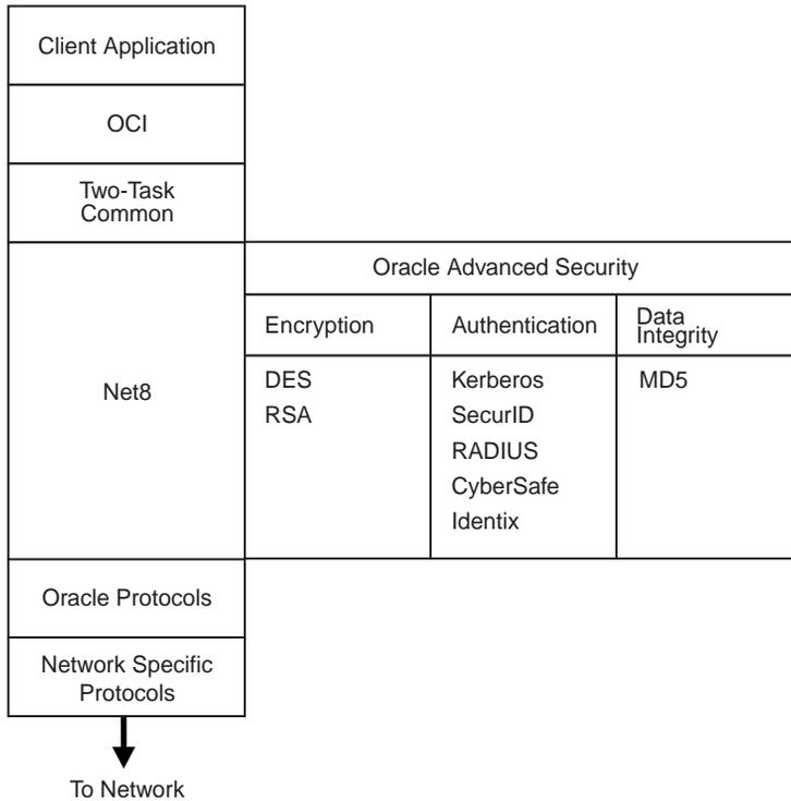
The Oracle Advanced Security option supports authentication through adapters that are very much like the existing Oracle protocol adapters. As [Figure 1–3](#) shows, authentication adapters integrate below the Net8 interface and allow existing applications to take advantage of new authentication systems transparently, without any changes to the application.
