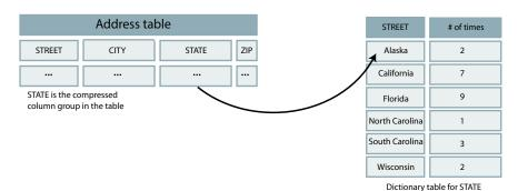
Figure 6-1 Column-Based Compression
