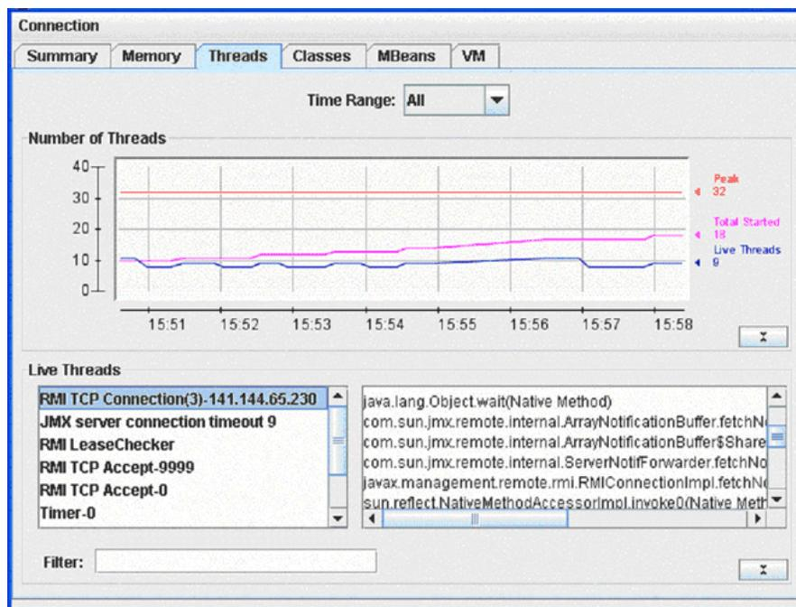
The chart on the Threads tab displays the number of live threads versus time, with a particular color representing a particular type of thread:
