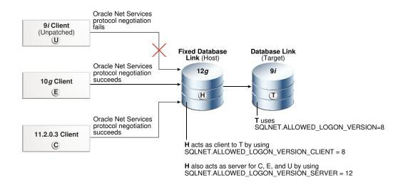
This scenario uses the following settings for the system that hosts the database link H:
