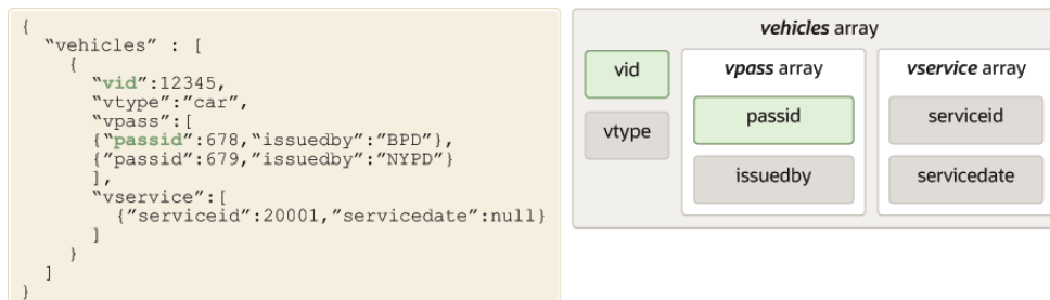
Figure 8-3 Composite Multikey Index
