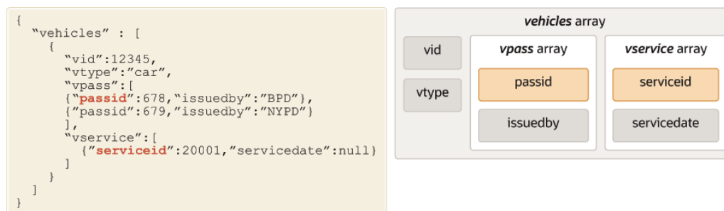
Figure 8-4 Composite Multikey Index (invalid)
