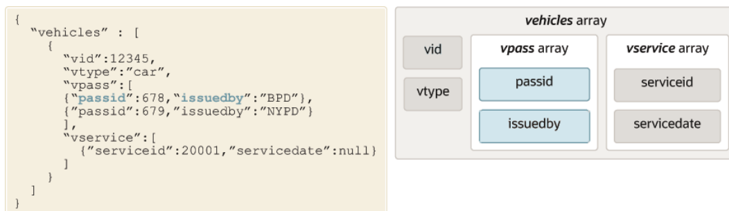
Figure 8-2 Composite Multikey Index
