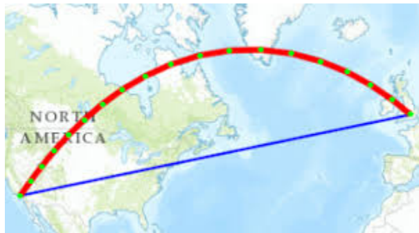
Figure 11-1 Geodetic vs Straight Line
