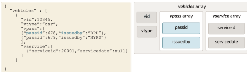
Figure 8-2 Composite Multikey Index
