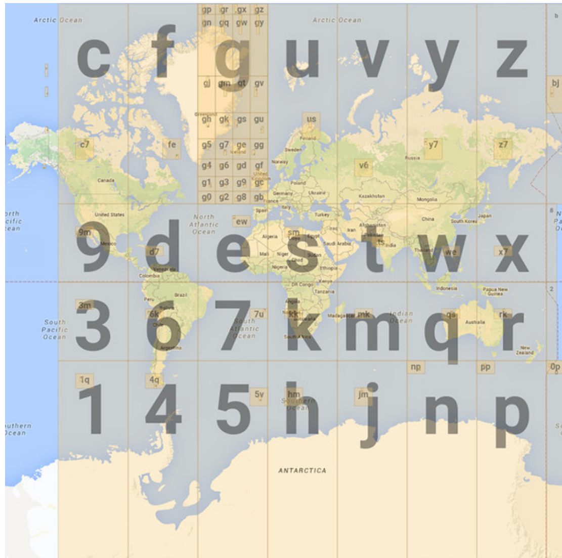
Figure 11-5 Level-1 and Level-2 Geohash Cells
