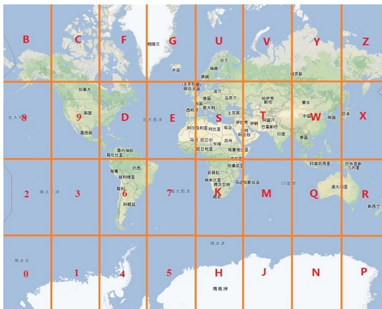
Figure 11-4 32 Level-1 Geohash Cells
