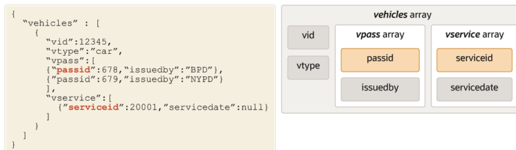
Figure 8-4 Composite Multikey Index (invalid)
