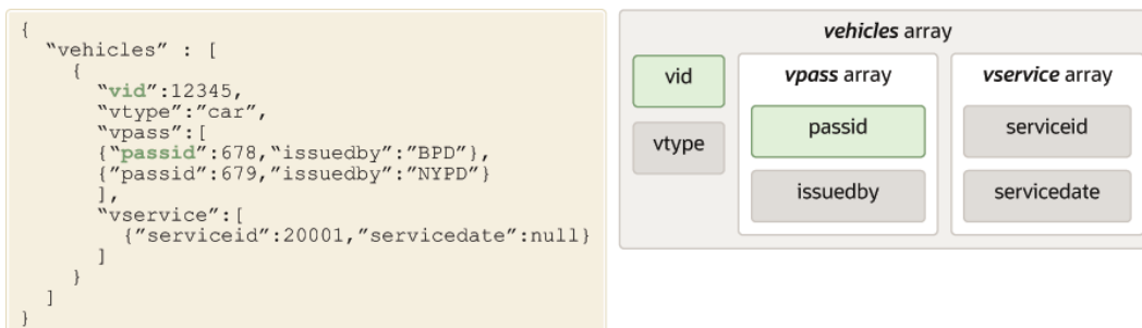
Figure 8-3 Composite Multikey Index
