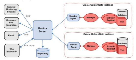
Schematic drawing of the Oracle GoldenGate Monitor topography showing how OGG Monitor server links external monitoring systems, the command line, email programs, and web browsers with GoldenGate instances. It also shows that GoldenGate instances are comprised of a monitor agent, a manager, and an extract/replicat component that leverages a trail and a database.
