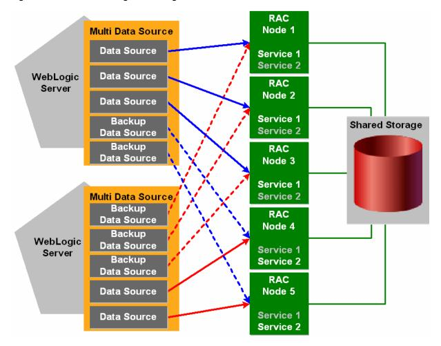
Figure C-4 Workload Management using Multi Data Sources
