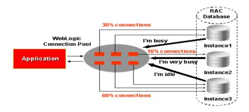
If FAN is not enabled, AGL data sources use a round-robin load balancing algorithm to allocate connections to Oracle RAC nodes.
