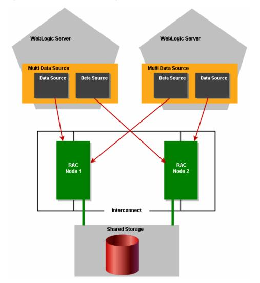
Figure C-2 Multi Data Source Configuration
