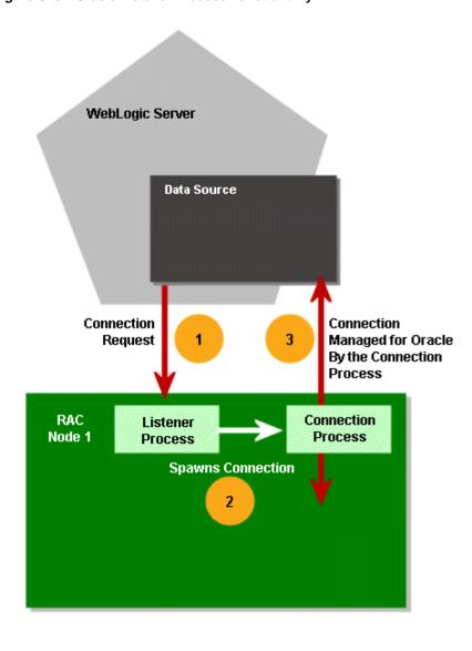
Figure C-3 Oracle Listener Process Functionality
