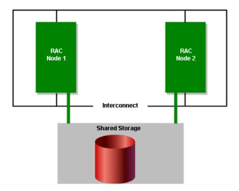
Figure C-1 Oracle Real Application Clusters Configuration
