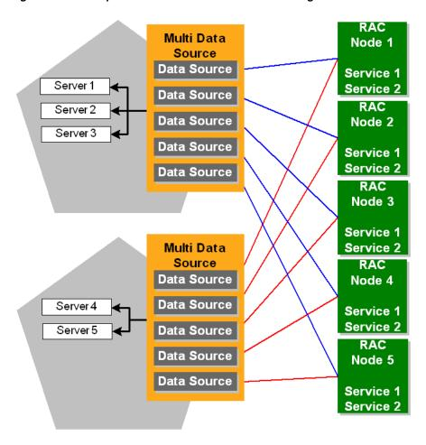
Figure C-6 Example multi data source Connection Configuration
