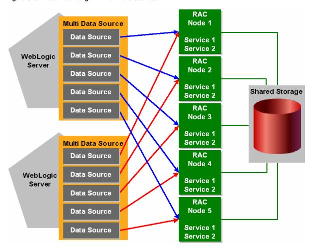
Figure C-5 Load Balancing with Multi Data Sources
