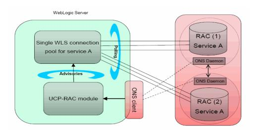
Figure 5-1 Active GridLink Data Source Connectivity
