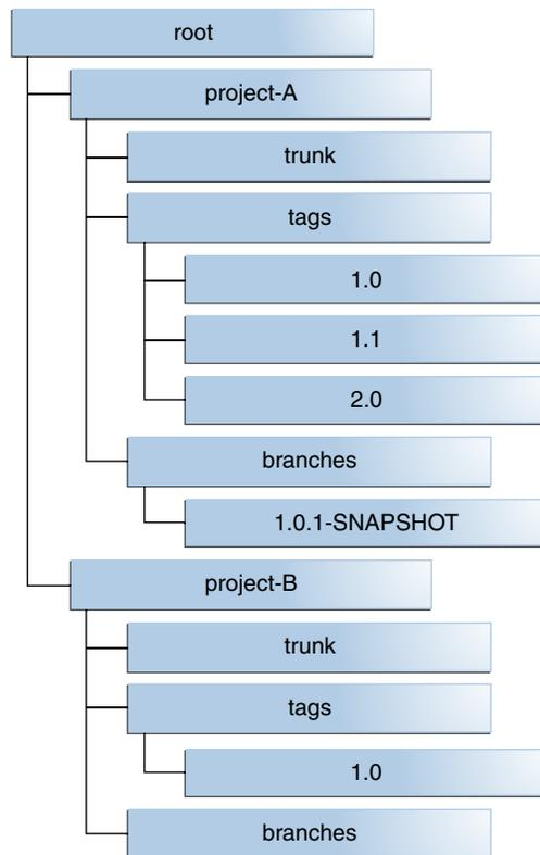
4. When the branch code fix is complete, the branch is copied from `project-A/branches/1.0.1-SNAPSHOT` to a `project-A/tags/1.0.1` tag. The release build can then be made from the tag.
