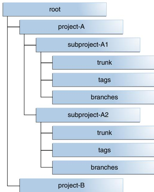
Development of the main code line occurs in the trunk directories. When a release is made, the current trunk source is copied into the tags directory, to a tag corresponding to the release. Subversion copy operations are not expensive in terms of storage because the server tracks changes internally.
