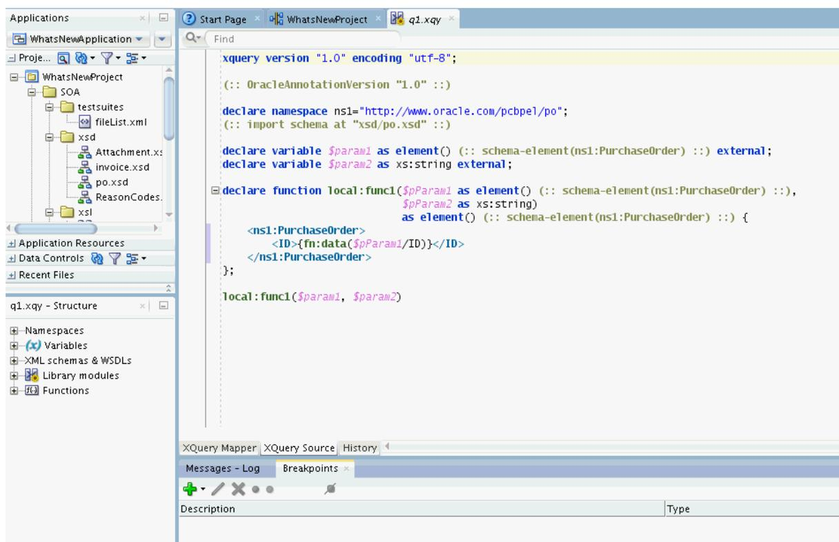
The XQuery source view provides code editing features like code highlighting, code completion, error highlighting, and code folding. You can also use Ctrl + click (click the left mouse button while holding down the Ctrl key) on a function name, variable name, schema, or schema element to navigate to the corresponding declaration for the function, variable, schema, or schema element respectively.
