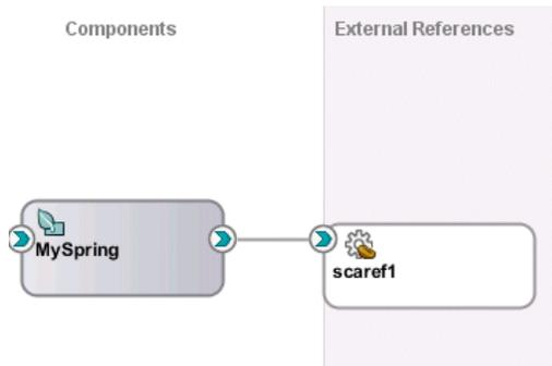
20. Double-click the EJB reference to display the automatically completed configuration, as shown in [Figure 55-13](#). The configuration details were created from the values you entered in the Insert Reference dialog in Step 11.
