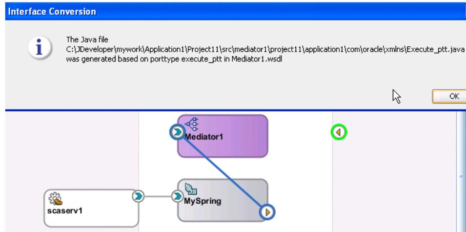
If you drag a wire between a Java interface and a WSDL-based component, and the WSDL file with the default name (based on the Java Interface name) already exists, you are prompted with four options. Click **Cancel** to cancel creation of the wire. [Figure 55-19](#) provides details.
