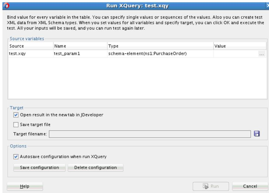
4. Specify values for all source variables that appear in the Source variables section. For simple data types, you can specify a value directly under the **Value** field. If your source variable uses a complex schema, click the ellipses (. . .) button to bring up the Edit Variable dialog. You can use an existing XML file to specify test data for the variable, or create an XML file with test data. Click Help for additional help with completing the Edit Variable dialog.
