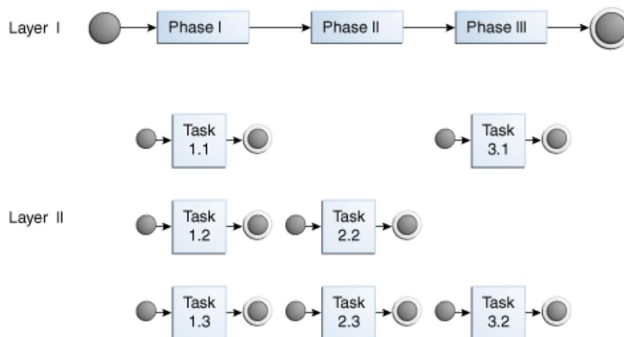
In [Figure 54-1](#), the phase I activity of the business process can delegate its work to one of the corresponding layer II processes: Task 1.1, Task 1.2, or Task 1.3.
