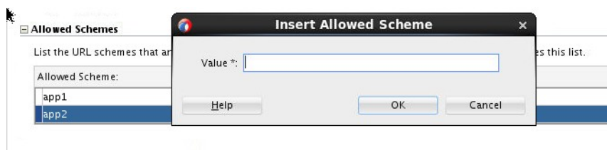
Figure 20-9 Registering a Custom URL Scheme that a MAF Applications Use to Invoke Another Application
