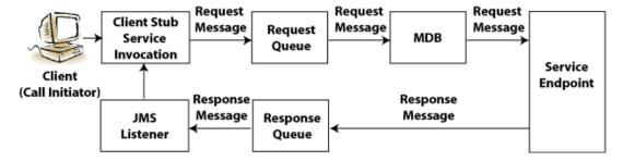
Figure 17–2 shows the flow of request and response messages for an asynchronous web service invocation using SOAP over JMS transport.
