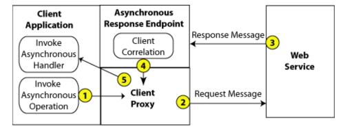
Figure 12–1 Asynchronous Client Transport Feature
