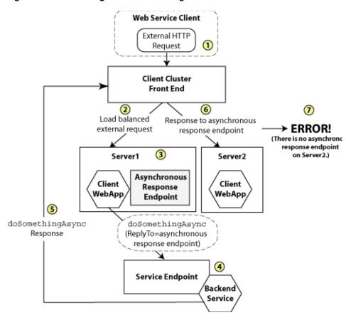
Figure 12–3 Clustering Scenario Resulting in an Error
