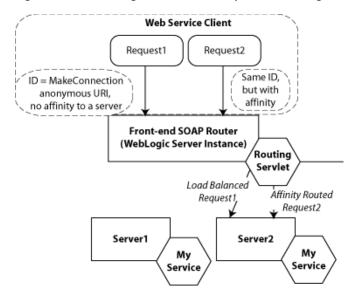
Figure 23–3 Routing Web Service Requests to a Single Server Using an ID
