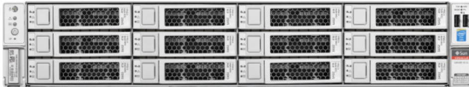
Figure B-1 Front View of Oracle Servers X6-2L and X5-2L
