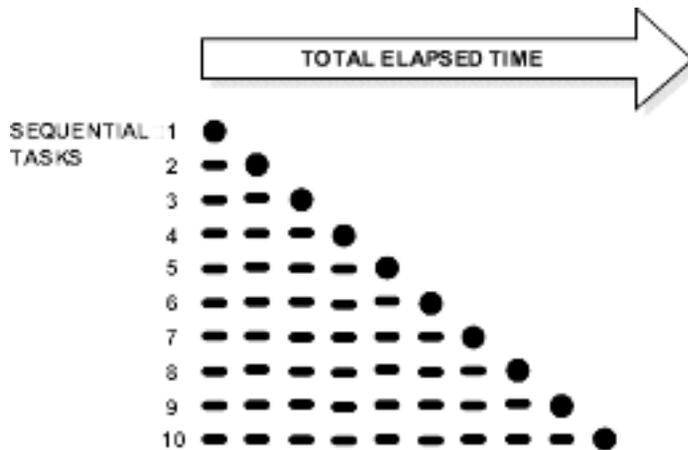
In this example, only task 1 runs without waiting. Task 2 must wait until task 1 has completed; task 3 must wait until tasks 1 and 2 have completed, and so on. (Although the figure shows the independent tasks as the same size, the size of the tasks will vary.)
