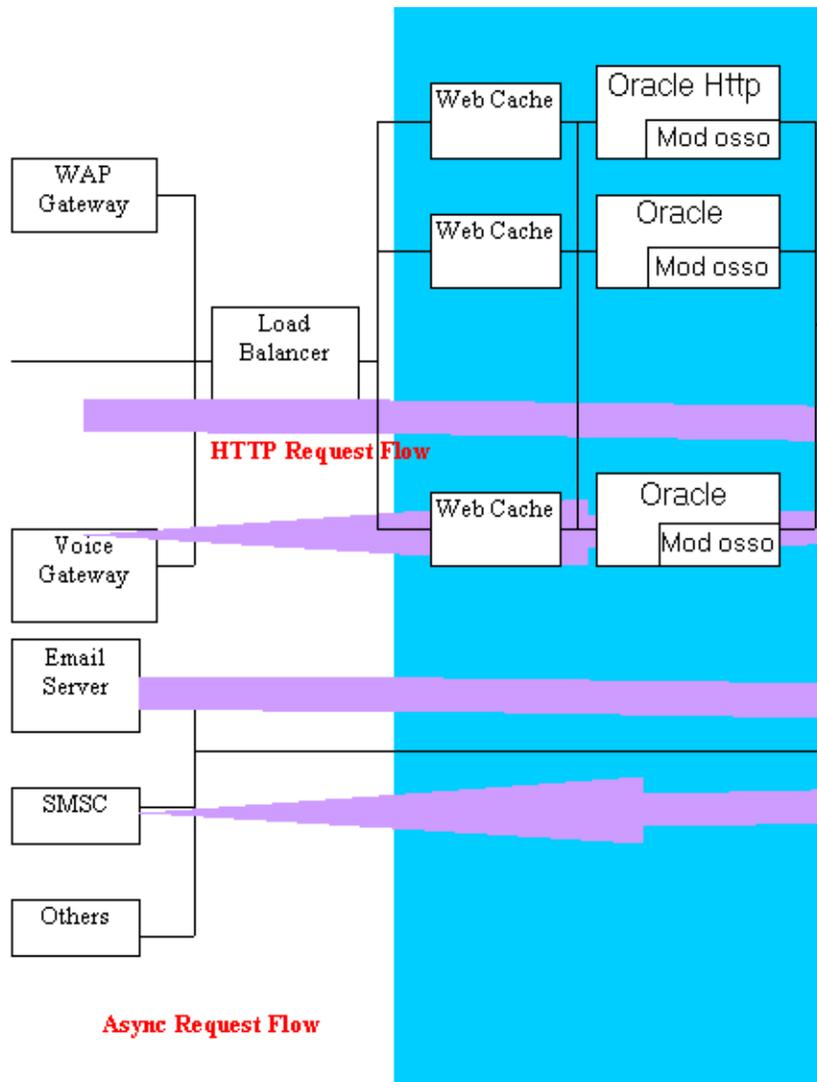
Figure 10-4 Oracle9iAS Wireless Process Architecture (part 2)
