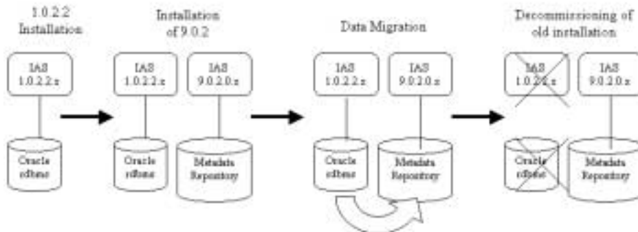
Figure 5-1 Overview of Repository Upgrade
