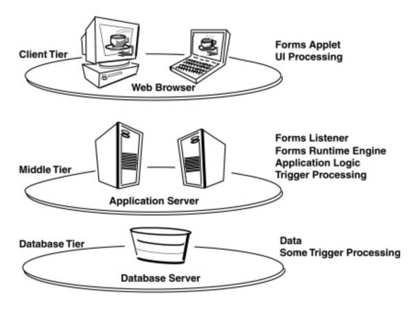
Figure 8–2 Forms Server Web-based architecture
