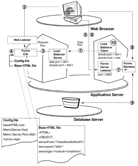
Figure 12–1 Forms Server load balancing
