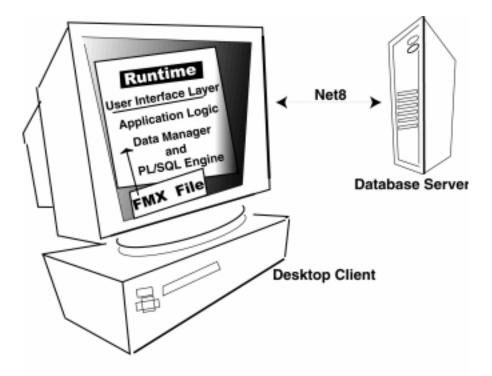
Figure 8–1 Forms Server client/server-based architecture
