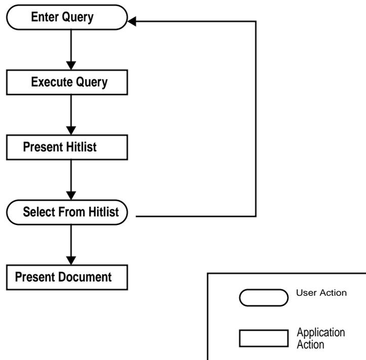
Figure 1–3 illustrates the flowchart of how a user interacts with a simple query application. The figure shows the steps required to enter the query and to view the
