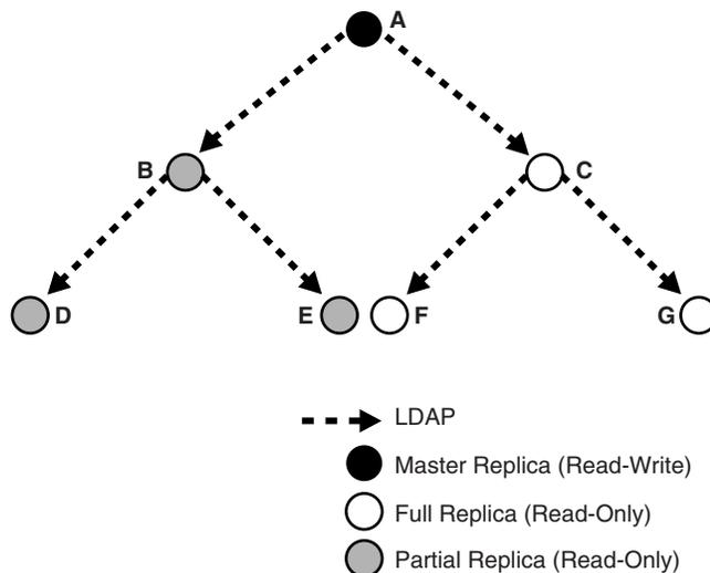
In fan-out replication, Oracle Internet Directory instances use the LDAP protocol to communicate with each other. The Select Oracle Internet Directory Replication Mode screen in the installer uses the term **LDAP Replication** to refer to fan-out replication.
