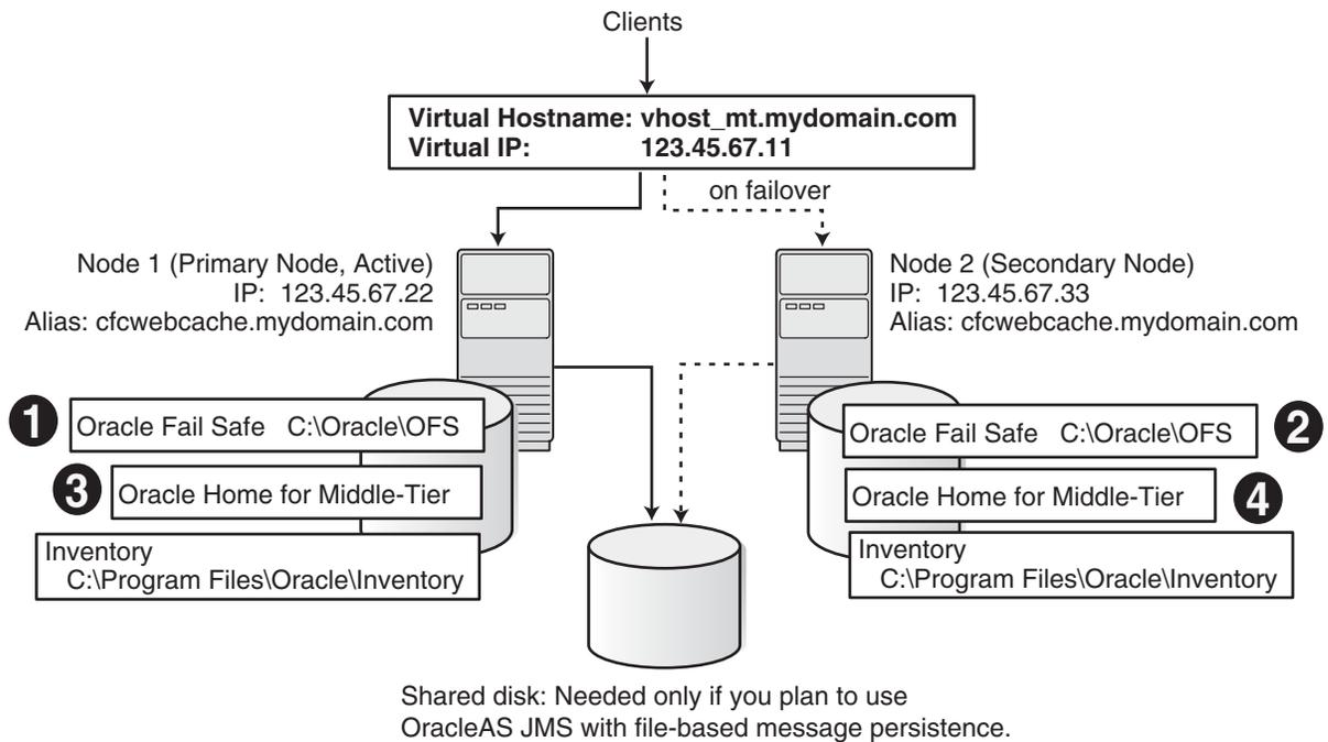
**Figure 10–27 OracleAS Cold Failover Cluster (Middle-Tier) Configuration with a Single Oracle Home****OracleAS Cold Failover Cluster (Middle-Tier) Configuration with a Single Oracle Home**
