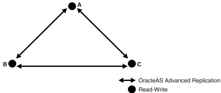
In multimaster replication, Oracle Internet Directory instances use the Oracle Database Advanced Replication protocol to communicate with each other. The Select Oracle Internet Directory Replication Mode screen in the installer uses the term **Advanced Replication** to refer to multimaster replication.
