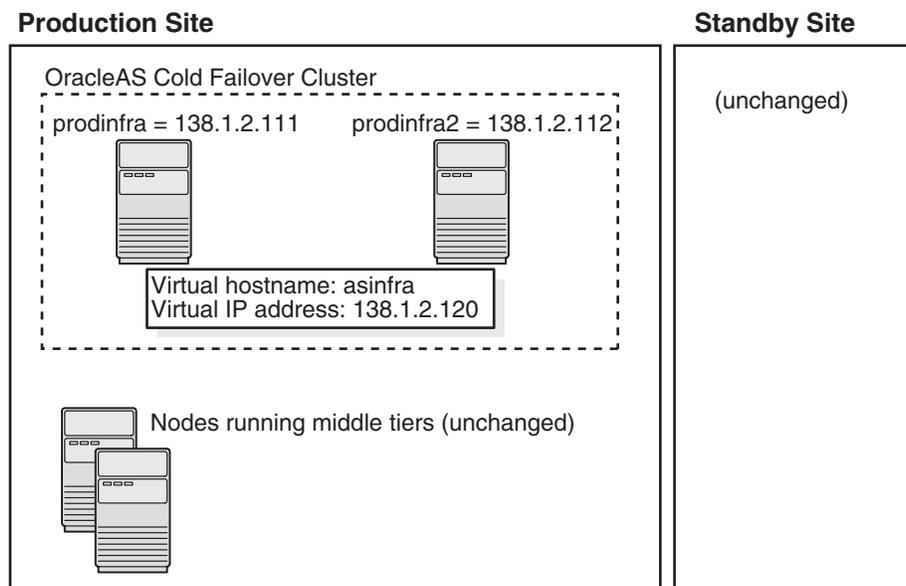
To set up OracleAS Cold Failover Cluster in this environment, use the virtual IP address (instead of the physical IP address) for asinfra.asha on the production site. The following example assumes 138.1.2.120 is the virtual IP address.
