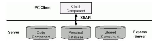
As shown in the figure, in this thin client configuration, the application programming interface (API) between the Financial Analyzer client component and the Financial Analyzer personal database using Express Server on the server is SNAPI (Structured N-Dimensional API).
