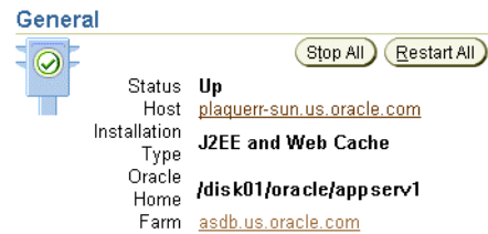
Figure 2–4 Using the General Section of the Application Server Home Page to Gather Information About the Oracle Application Server Environment
