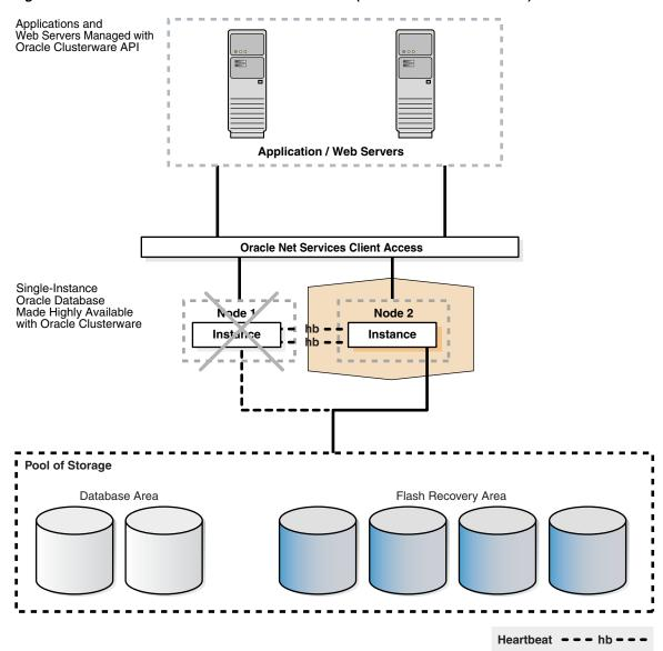
Figure 4–3 Oracle Database with Oracle Clusterware (After Cold Failover Cluster)
