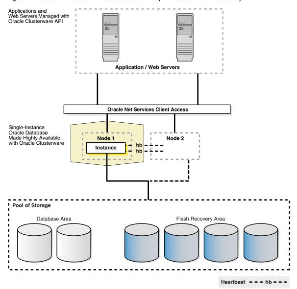
Figure 4–2 Oracle Database with Oracle Clusterware (Before Cold Failover Cluster)
