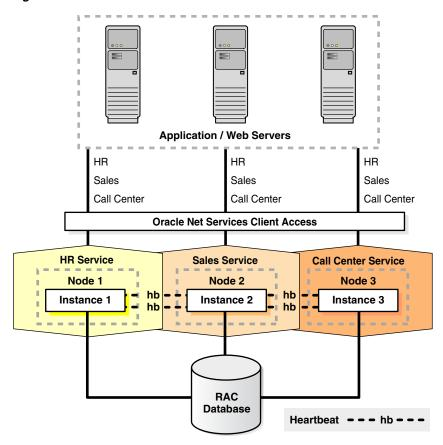
Figure 4–4 Oracle Database with Oracle RAC Architecture
