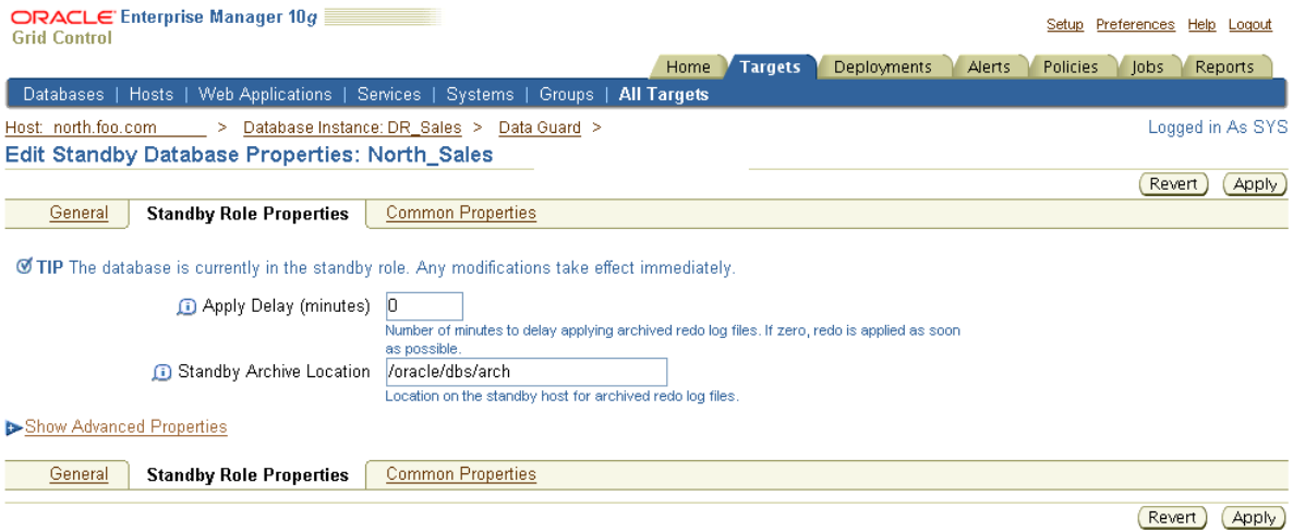
Figure 6–26 Standby Role Properties
