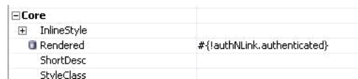
Figure 10-43 Setting the Rendered Property Based on the Authenticated State of the User
