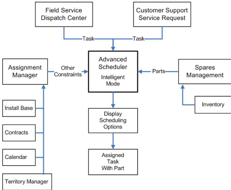
Advanced Scheduler receives unassigned tasks created in either the Field Service Dispatch Center or the Customer Support Service Request window. The dispatcher selects a task to be scheduled.
