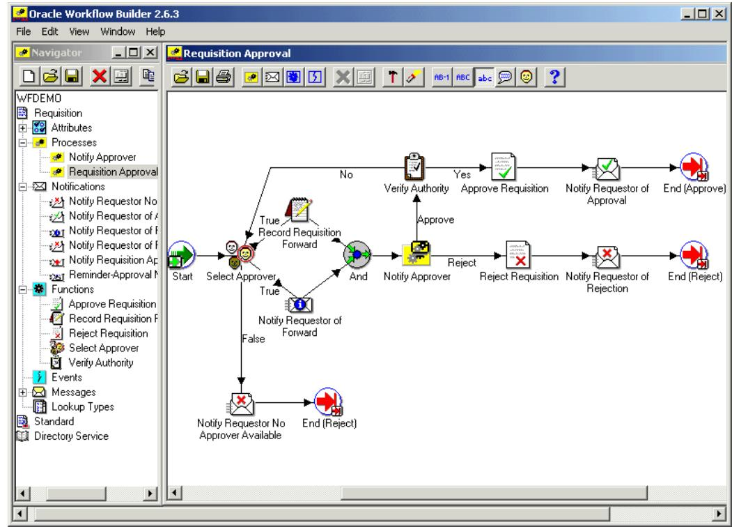
We refer to the whole drawing as a process or process diagram. The icons represent activities, and the arrows represent the transitions between the activities. In the above example, new items are created for the process when a user creates and submits a requisition in the appropriate application.
