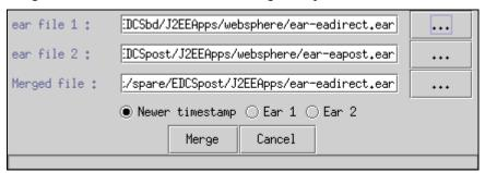
You can click on the ... button to bring up a file dialog to locate the EAR files. Be sure to select which method to use when merging the EAR files. The example shows EAR 2 as the selected method, which means the eareapost.ear file's contents will override any entries in EAR 1.
