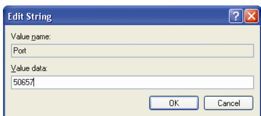
Figure 9-11: Setting the string value for the port
