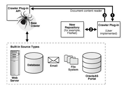
Two interfaces in the Crawler Plug-in API (CrawlerPluginManager and CrawlerPlugin) need to be implemented to create a crawler plug-in. A crawler plug-in does the following:
