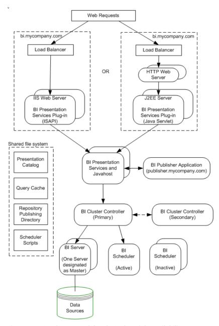
Figure 4. Deployment of Oracle BI for High Availability
