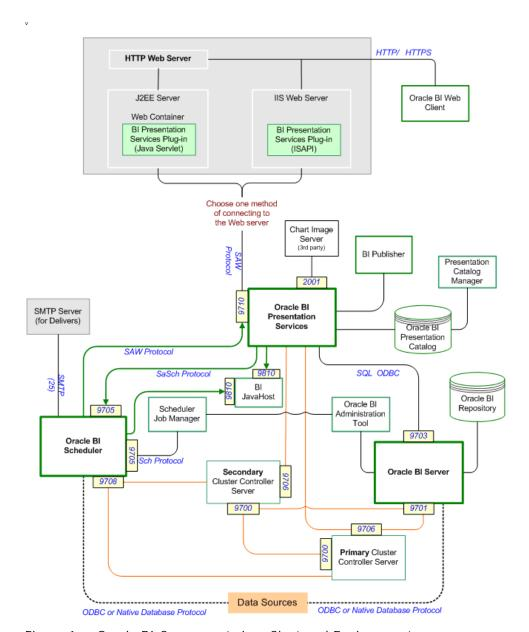
Figure 1. Oracle BI Components in a Clustered Environment
