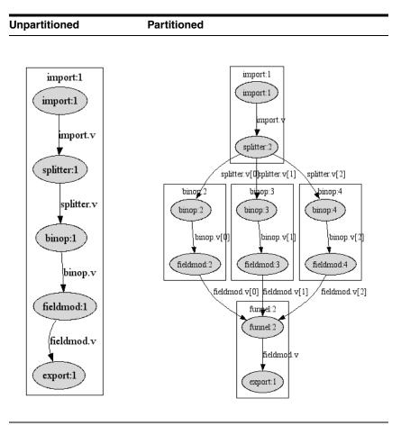
In this example, the SPLITTER operator is the partitioner. It distributes the records read by the IMPORT operator across three partitions. The BINOP and FIELDMOD operators are duplicated across all three partitions by RETL. Finally, a funnel is inserted before the EXPORT operator, to gather the partitioned records back into one dataset.
