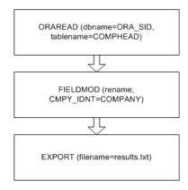
In this flow diagram, several attributes are also shown to give more information about what exactly this flow does. This flow pulls the COMPHEAD table out of the ORA\_ SID database (using the ORAREAD operator), renames the column CMPY\_IDNT to COMPANY (using the FIELDMOD operator), and exports the resulting records to the file results.txt (using the EXPORT operator).
