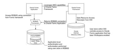
Figure 8–2 outlines the interaction between the Oracle Forms Framework, OID, and the actual Forms Application.
