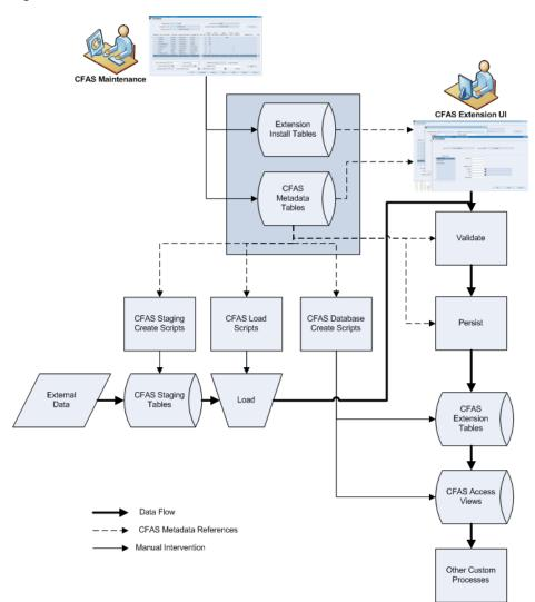
Figure 1–2 CFAS Data Flow
