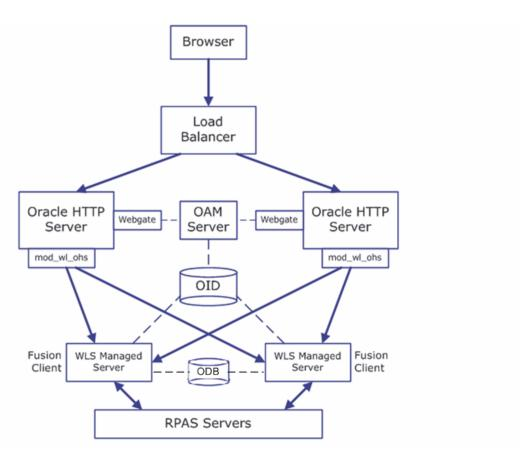
Figure 5–2 Load Balancer for an SSO Deployment
