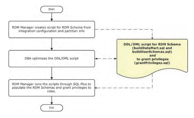
Figure 8-3 Installation: Building the RDM Schemas - Alternative Process
