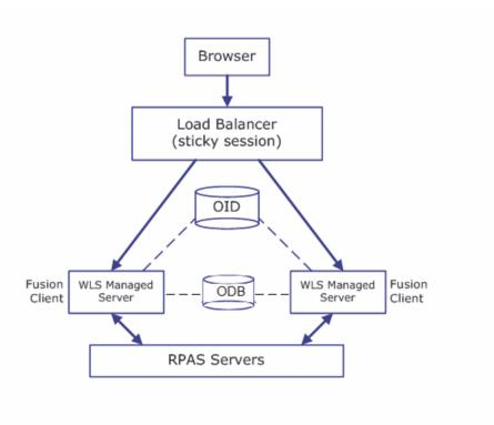
Figure 5–1 Load Balancer for a Non-SSO Deployment
