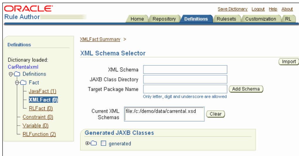
Figure 4-6 Rule Author Definitions XML Schema Selector After Adding XML Schema
