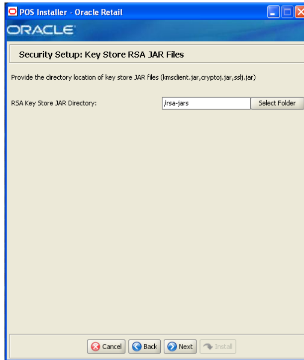
Figure B-27 Security Setup: Key Store JAR Files for RSA Key Manager 3.0
