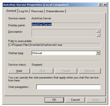
Once the Service has been started, it behaves exactly as if run in "non-service" mode. The AutoVue server icon appears in the System Tray. To stop the service click **Shutdown**.
