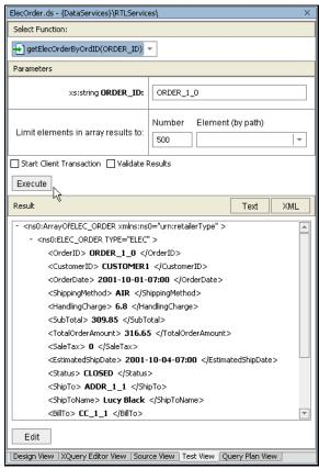
Figure 7-6 Executing a simple parameterized query
