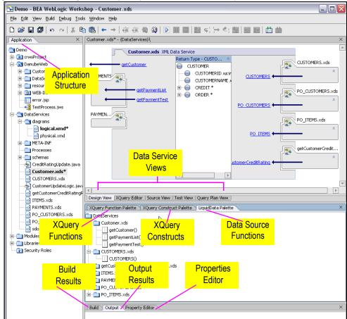
Figure 2-5 Some WebLogic Workshop Components in a DSP-based Project
