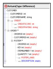
The arrows to the left of changed items indicate whether the change is originating locally in the return type ( $\rightarrow$ ) or in the data service's XML type (<-).
