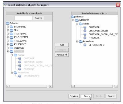
Figure 3-11 Selecting Stored Procedure Database Objects to Import
