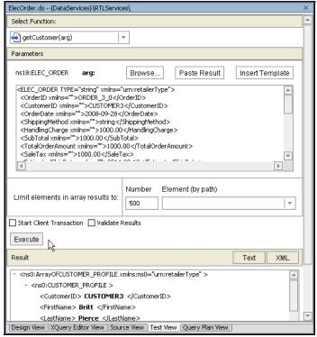
Figure 7-9 Using XML Type Template to Guide Data Input
