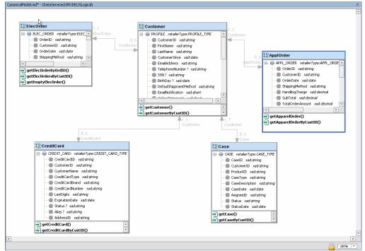
Figure 5-1 Model Diagram of Physical Data Services
