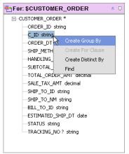
In Figure 6-22 output will be grouped by the C\_ID (customer ID) element. Once a GroupBy node is created, mappings to target objects — such as the return type — are done through the new node.
