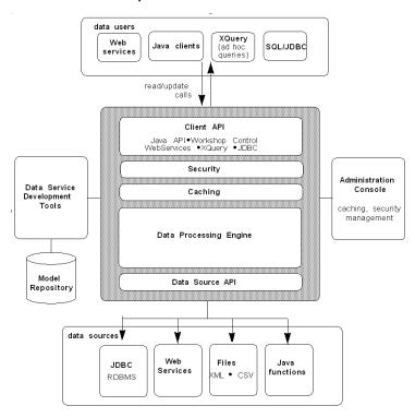
Figure 1-2 Data Services Platform Component Architecture
