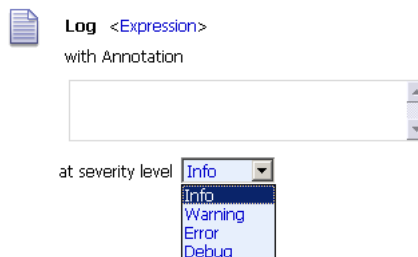
Figure 18-34 Log Action Configuration Parameters
