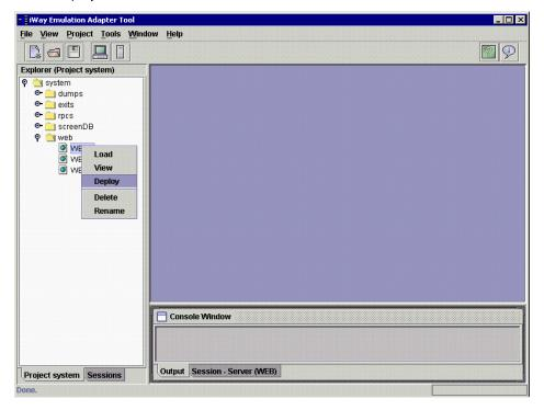
Selecting Deploy automatically transfers the Web components created by the Telnet Designer to the supplied Web application server. The following events occur:
