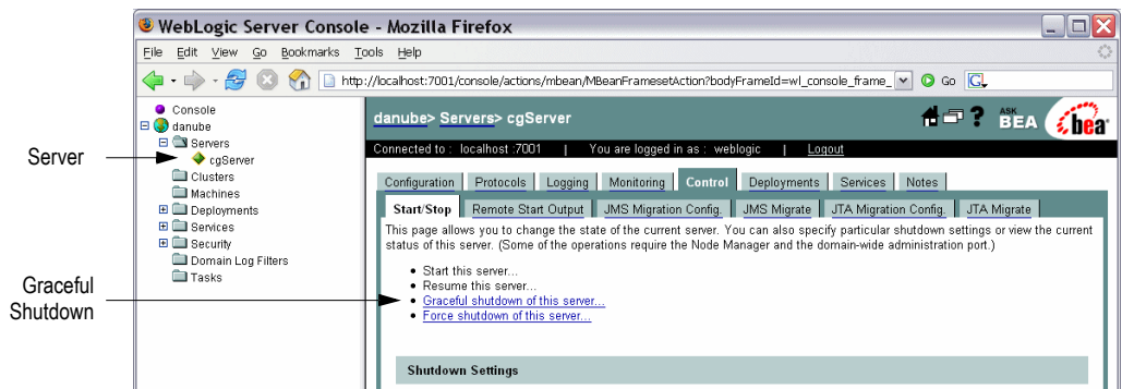
Figure 2-3 Graceful Shutdown of a Server
