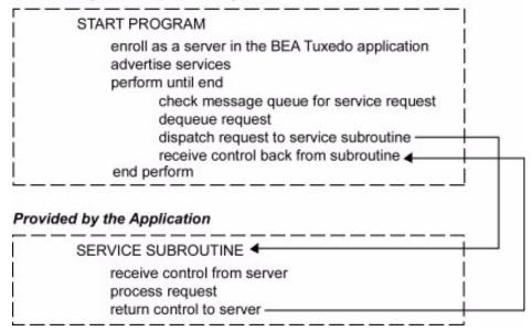
After initialization, an ATMI server allocates a buffer, waits until a request message is delivered to its message queue, dequeues the request, and dispatches it to a service subroutine for processing. If a reply is required, the reply is considered part of request processing.
