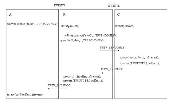
In the preceding example, service B is a member of a conversation that has initiated a connection to a second service called C. In other words, there are two active connections: A-to-B and B-to-C. If B is in control of both connections, a call to tpreturn() has the following effect: the call fails, a TPEV\_SVCERR event is posted on all open connections, and the connections are closed in a disorderly manner.
