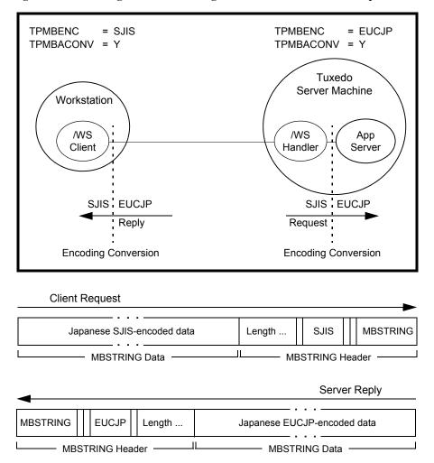
Figure 3-1 Encoding Conversion Using MBSTRING Buffers—Example
